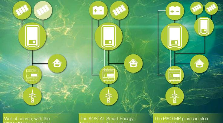
Well of course, with the PIKO MP plus – featuring one or two MPP trackers. The KOSTAL Smart Energy Manager can be used to connect a battery and therefore store energy. The PIKO MP plus can also be connected to an existing PV system on the AC side only, where it is used to store energy.
