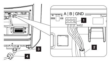
Fig. 26: Connection for digital energy meter (Modbus RTU)
