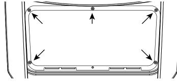
Fig. 20: Taking off terminal compartment cover
