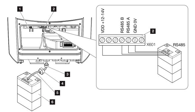
Fig. 30: Battery connection for RS485 communication
