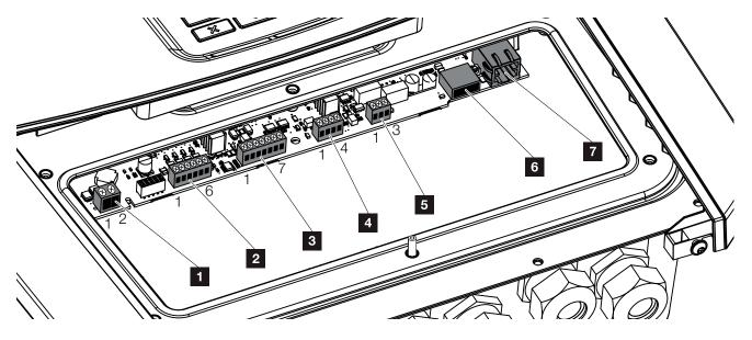
Fig. 24: Smart Communication Board - interfaces
