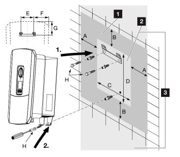
Fig. 16: Wall mounting with wall mount
