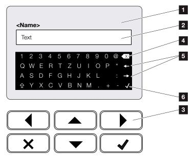
Fig. 36: Using keyboard to operate the display
