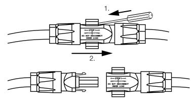
Fig. 33: Disconnecting SUNCLIX DC plug
