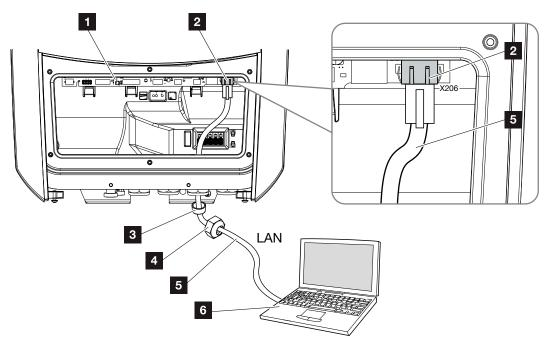
Fig. 28: Connecting battery inverter and computer with an Ethernet cable
