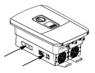
Signs and labels are attached to the housing of the battery inverter. These signs and labels may not be altered or removed.
