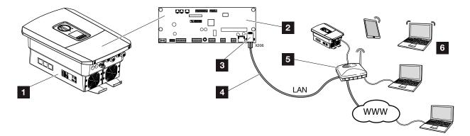
Fig. 27: Communication connection
