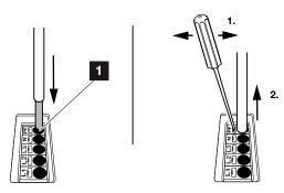
Fig. 22: Spring-loaded terminal strip
