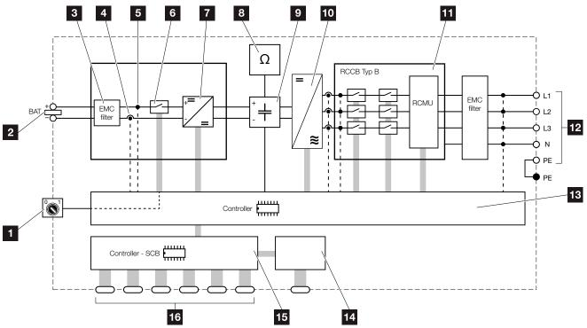
Fig. 57: Block diagram
