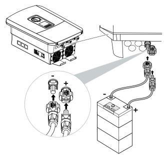
Fig. 32: Battery's DC connection
