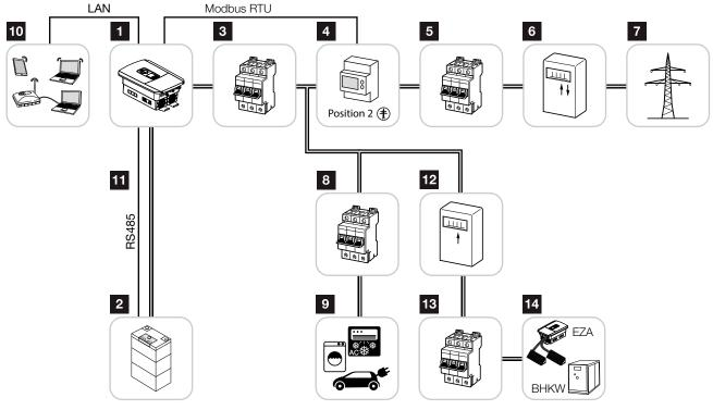
Fig. 7: Battery inverter with battery connection
