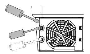
Fig. 53: Loosen fastening straps
