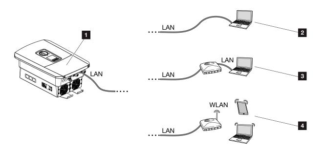
Fig. 42: Connection from computer to battery inverter
