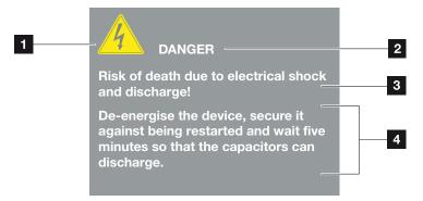
Fig. 4: Structure of the warnings
