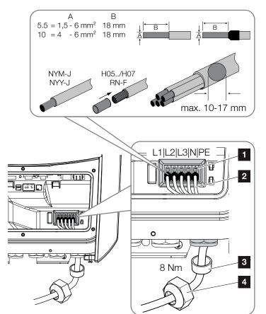
6. Correctly lay the mains cable from the power distributor to the battery inverter.
