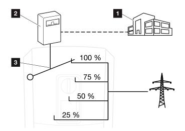
Fig. 50: External battery control via digital inputs
