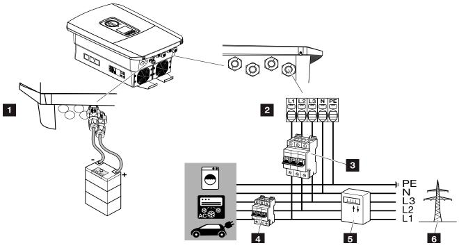
Fig. 18: Overview of electrical connections
