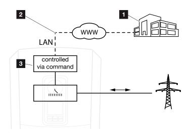
Fig. 49: External battery control via Modbus (TCP)
