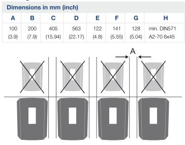
Fig. 17: Wall mounting of several battery inverters
