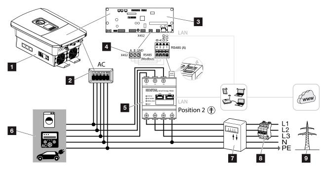
Fig. 25: Wiring diagram for energy meter - grid connection (position 2)
