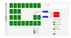
To create a map of the system that matches the physical layout\*, remove the peel-off stickers from the TS4 covers or record the barcodes on a map that represents their physical location.
