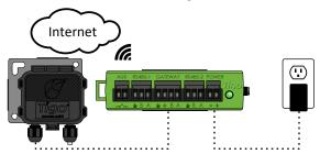
The Cloud Connect Advanced (CCA) requires AC power, an Internet connection (Ethernet or Wi-Fi), and an RS485 communication cable connection to the TAP(s).
